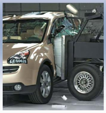
How vehicles are evaluated in front, side, and rear tests: The Institute's frontal crashworthiness evaluations are based on results of frontal offset crash tests at 40 mph. Each vehicle's overall evaluation is based on measurements of intrusion into the occupant compartment, injury measures recorded on a Hybrid III dummy positioned in the driver seat, and analysis of slow-motion film to assess how well the restraint system controlled dummy movement during the test.
